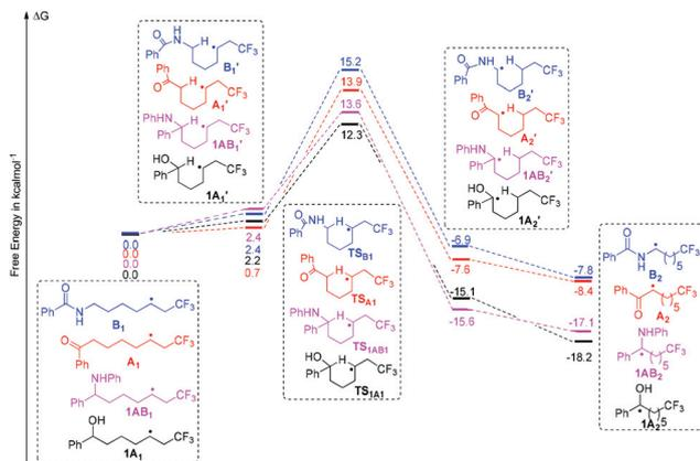
**Scheme 5** Energy profiles for the 1,5-HAT process calculated at the M06L/6-311G\* level of theory.
